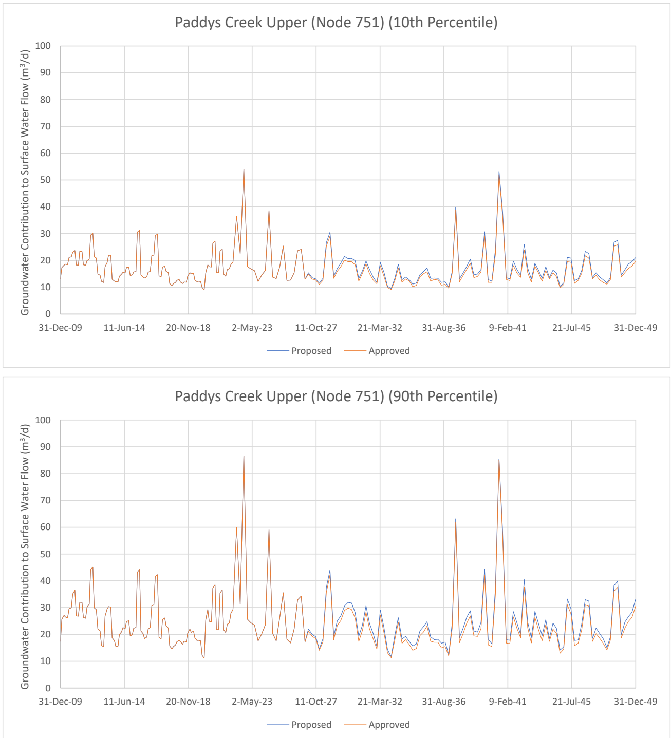
Figure 4-85: Modelled Groundwater Contribution to Surface Water – Prediction Simulation (Stochastic): Paddys Creek Upper (Node 751)
